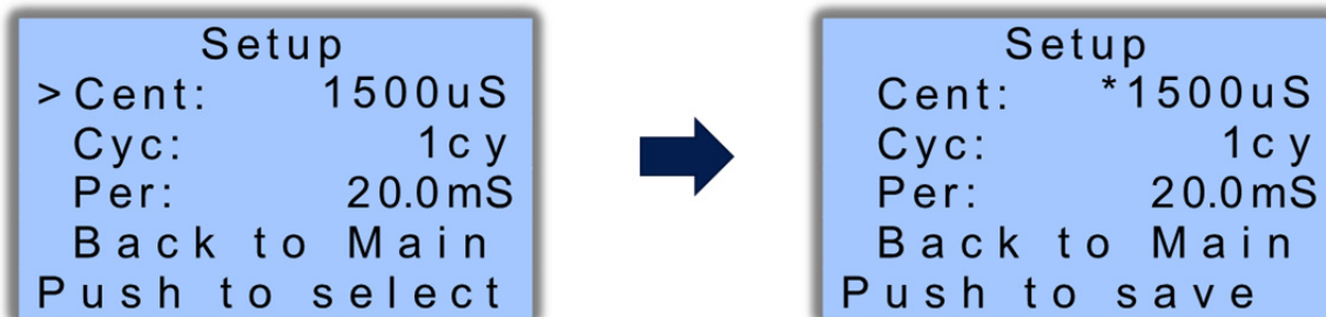
FIGURE 8 – Setup menu and options selection; note the asterisk (*) next to the value to be changed
